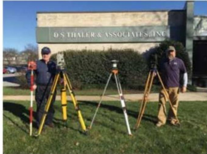
The author holding a Range Pole with a reflective prism and from left: a Total Station, a GPS Receiver and a Transit. Surveyors generally used transits and steel tapes from the early part of the 20th century until about 20 years ago when they were largely replaced by Total Stations (which are electronic distance and angle measuring instruments) and GPS.
